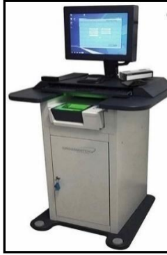
Image No 1: a Livescan optical fingerprint scanner
